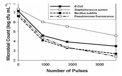
Hence to make this process more effective high electric field of range 85-90 KV/cm should be applied, capacitor of range 300-400 nF should be used and medium conductivity should be reduced.
